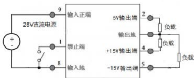
Figure 8. Connection diagram of BSTHF28 series products
